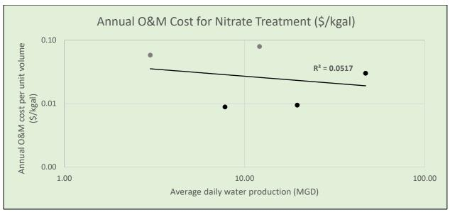
Figure 9: Average annual O&M cost per unit volume plotted against average annual water production. Both axes are log-transformed. Data from the study locations are highlighted in black.
